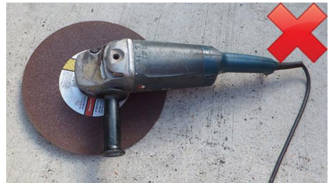
Angle grinder with no guard
